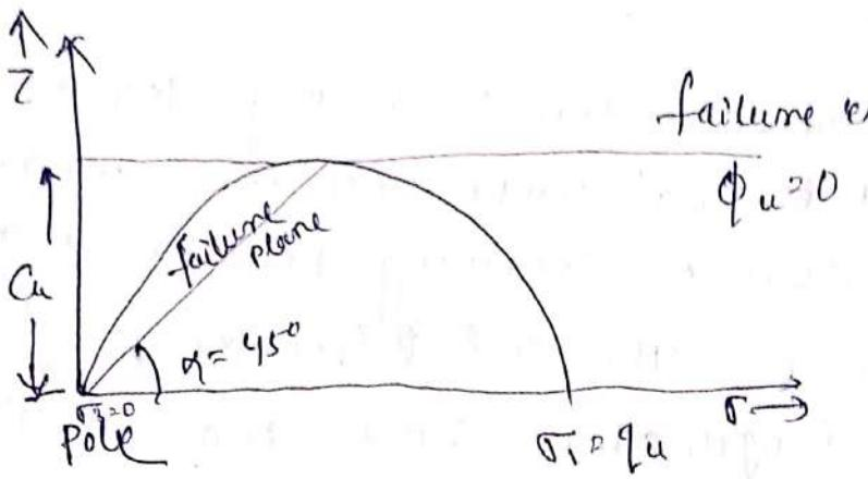
The Undrained shear strength parameters obtained are denoted by  $C_u$  and  $\phi_u$ .
